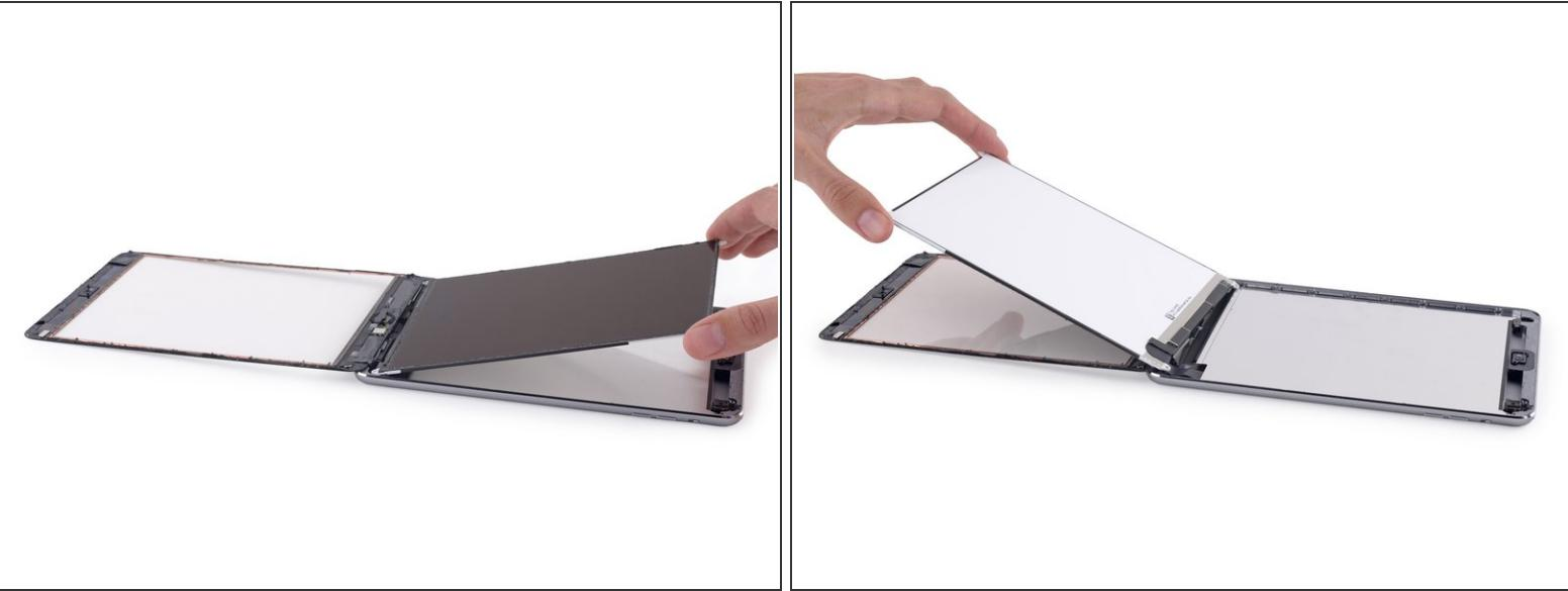
**⚠** Do not attempt to fully remove the LCD. It is still connected to the iPad by several cables at the home button end. Lift only from the front-facing camera end.
